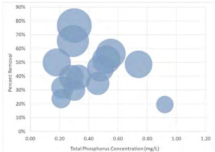
Figure 1 shows the effectiveness of Hydrestor® media to remove on average 39% Total Phosphorus at various low level concentrations.
